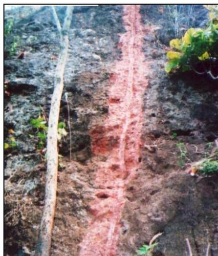
Channel sampling on the scarp section of Bauxite plateau
